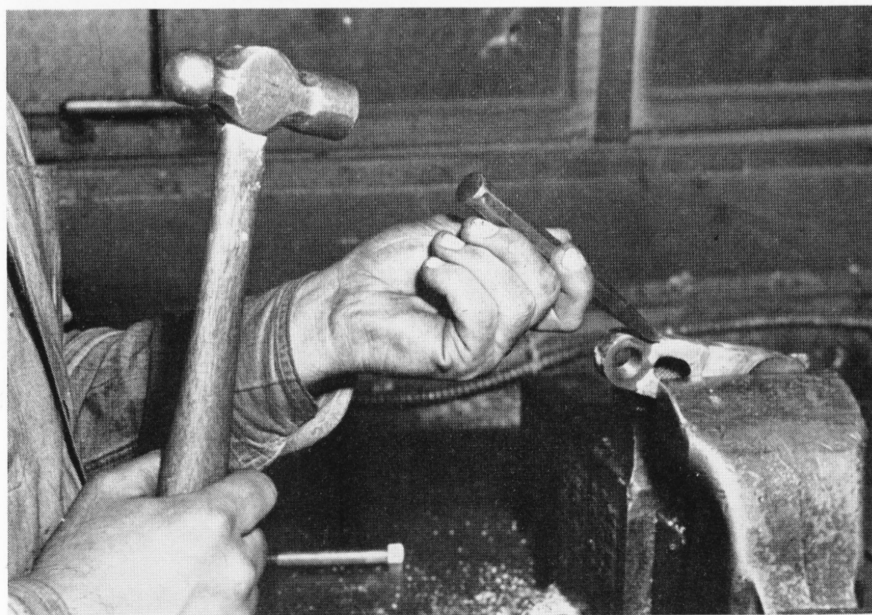
Many employees of late, turning up at the hospitals with skinned knuckles, all gave a similar answer—"The chisel slipped and WHAM." There is a way of defeating slipping tools of this type as illustrated above. By holding the tool from beneath, the hand does not follow the path of the chisel or drift if it slips. Held from the topline, a slipping chisel means that the hand will hit against the immovable object. Unfortunately, the knuckles bear the brunt.
